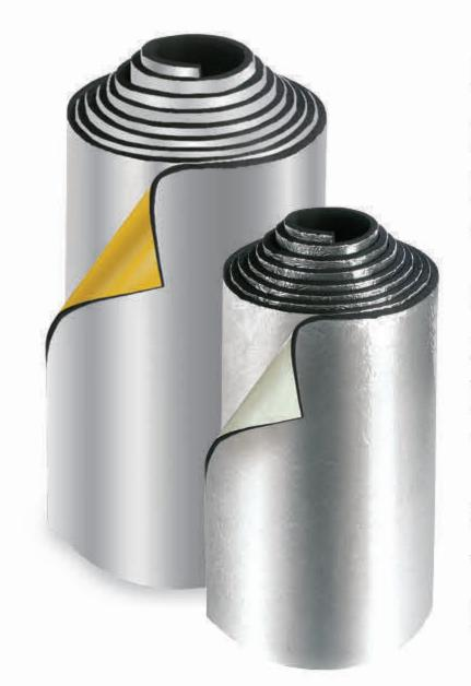
ISOROLLS TC UV PLUS with three layer protective film, of polyester, aluminum and polyethylene, total thickness of 99 µm, with resistance of at least five (5) years to solar radiation of Mediterranean climate zone, from -40°C to +100°C and longitudinal tensile strength of 75N and 78N transverse, according to DIN 55531, also certified according to requirements of the EN14304 standard.
