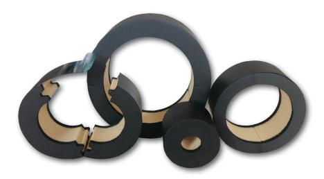
**ISOCLAMPS** are used to eliminate insulation gaps and reduce the possibility of thermal bridge creation, during the support of the insulated tubing (made by collar or metal bracket), in refrigeration or heating installations. They are suggested for applications where the temperature is between  $-45^{\circ}$ C to  $+105^{\circ}$ C.
